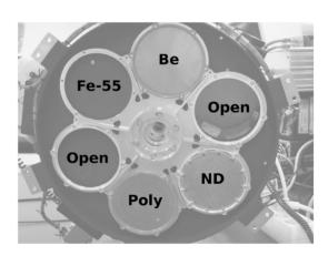
**Fig. 10** Filter selection. The filter wheel has three filters, two open positions, and one position with a radioactive Fe-55 calibration source. The three filters are Beryllium filter (Be), neutral-density filter (ND), and polyimide filter (Poly).
