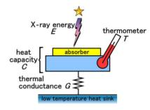
**Fig. 6** Concept of X-ray micro-calorimeter
