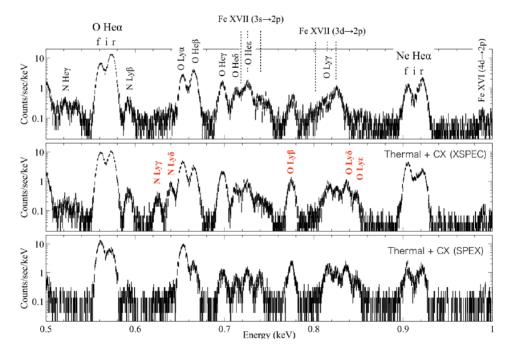
**Fig. 23** 30-ks simulated Resolve spectra of a shell region of the Cygnus Loop. Top: Assumed model is a typical thermal plasma with electron temperature of 0.2 keV. Middle: Same as the top panel but added a charge-exchange model in XSPEC. Bottom: Same as the middle panel but simulated in SPEX with similar model parameters.
