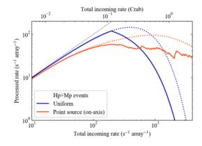
**Fig. 9** Incoming vs. processed rate for Hp+Mp events (solid). Because of the limitation in the CPU load ("PSP limit"), the processed rate is reduced from what would otherwise be observed (dotted). The calculations do not include the effect of electrical crosstalk.
