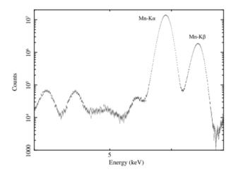
**Fig. 12** 55 Fe Spectrum of a FM CCD chip in a ground calibration.
