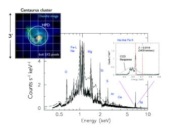
**Fig. 7** Pixel layout (upper left panel). The array encompasses ∼74% of photons of a point source at the center. Simulated spectrum of Centaurus cluster (bottom left).
