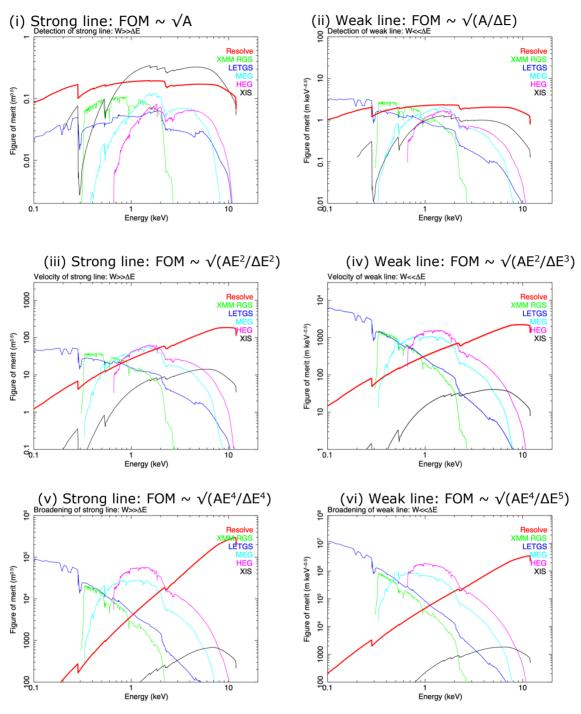
**Fig. 17** Figures of merit (FOM) for (i) detection of strong line, (ii) detection of weak line, (iii) velocity of strong line, (iv) velocity of weak line, (v) broadening of strong line, (vi) broadening of weak line. Strong lines are defined here as lines with equivalent width W larger than the instrumental resolution  $\Delta E$ , weak lines have W smaller than  $\Delta E$ .
