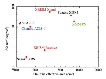
**Fig. 19** Grasp vs on-axis effective area at 7 keV of Resolve and Xtend. Suzaku XIS, Chandra ACIS-I, XMM PN are also shown for comparison. The grasp is defined as the product of field of view and effective area.
